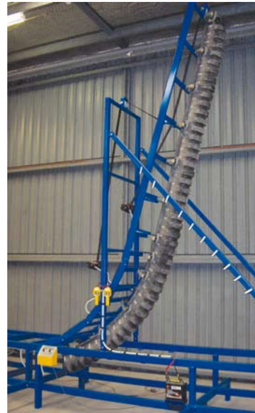
A prototype of the ICSI conveyor operating at an 80-degree angle.
