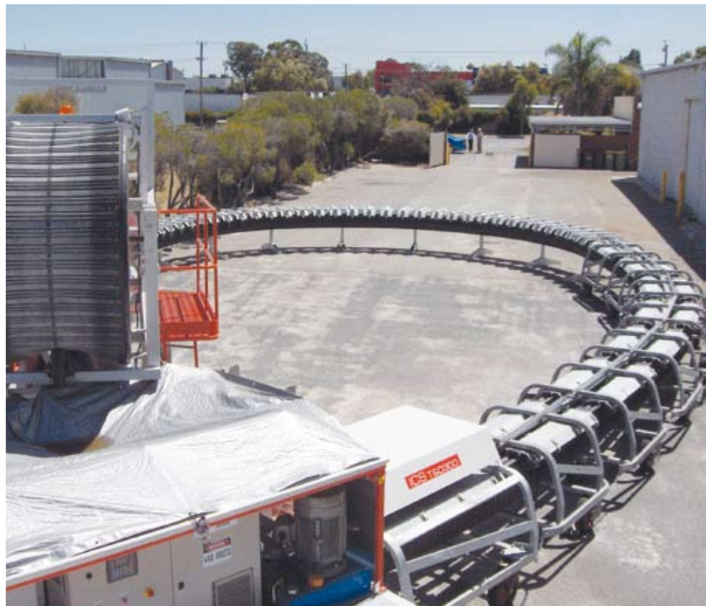
Above left: ICSI managing director Michael Pietsch and a working version of the system. Note how the belt opens out to discharge. Above right: The conveyor system is capable of handling turns with a 5m radius.
