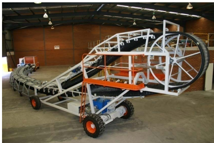
Figure 10: A completely mobile ICS that can be moved as an entire unit via remote control
