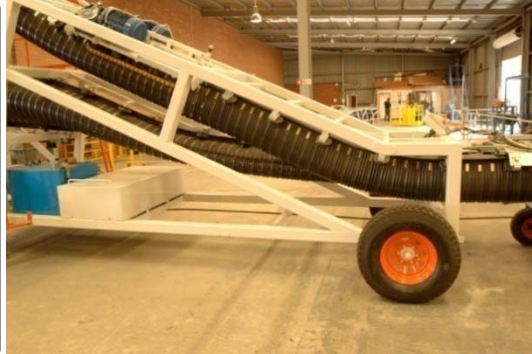
Figure 9: Transition from horizontal to vertical within a 4m radius for 300mm diameter belt
