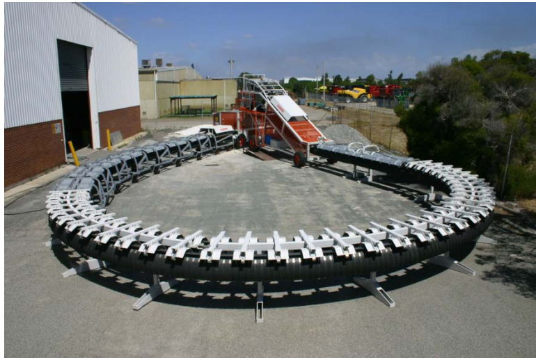
Figure 7: ICS test unit utilising 300mm belt negotiating a 5 metre radius
