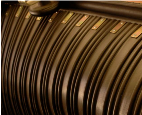
Figure 1: Belt displaying typical corrugations patterns
