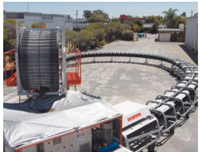
The conveyor system is capable of handling turns with a 5m radius thanks to a corrugated belt design that allows the belt to “flex”.
