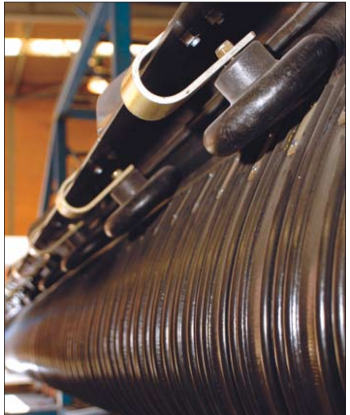
The Innovative Conveying System is an enclosed conveyor that uses a patented corrugated belt to allow flexibility in both the horizontal and vertical directions. The belt is supported on custom designed idler assemblies.
