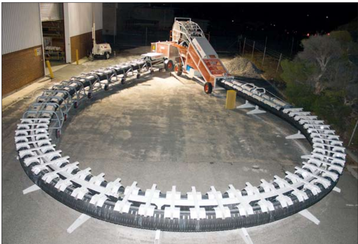
The in house test unit negotiating a radius of five metres through 270 degrees.
