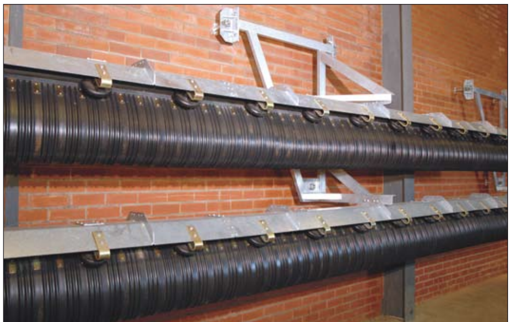
The Innovative Conveying System can be mounted on a variety of custom built brackets. The load and return strands can be side by side, one on top of the other or can follow completely independent paths. This configuration was developed for mounting on the side of mining declines or to the wall of a tunnel.
