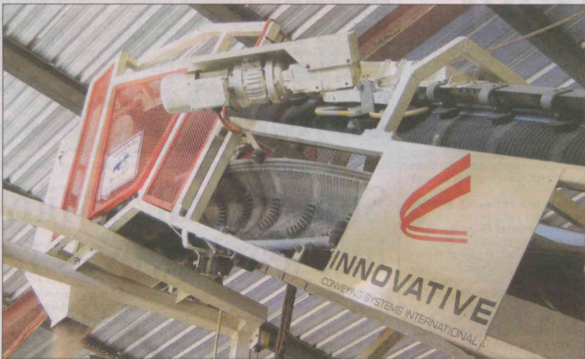
Better belts: ICS uses an enclosed system made of polyurethane that can carry materials at steep angles.
